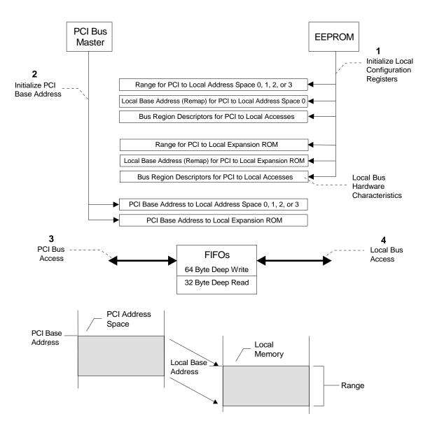
Figure 3-1. PCI Master Direct Access of Local Bus
