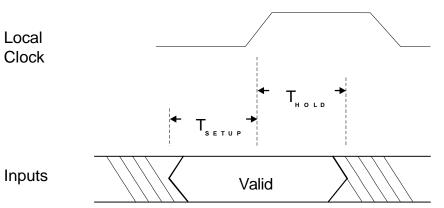
Figure 6-2. PCI 9050 Local Input Setup and Hold Waveform
