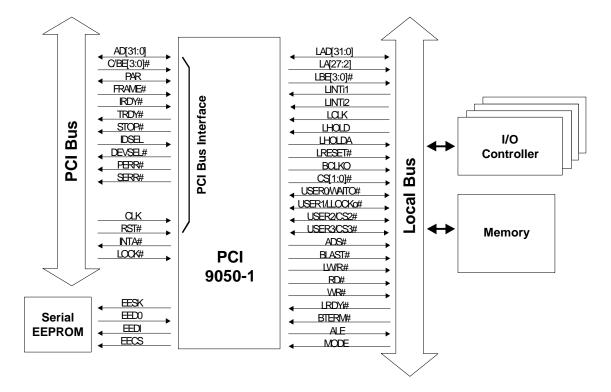
Figure 1-1. PCI 9050-1 Block Diagram
