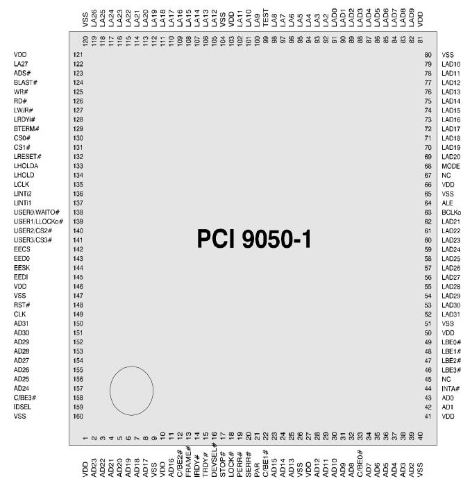
Figure 7-3. PCI 9050-1 Pin Out
