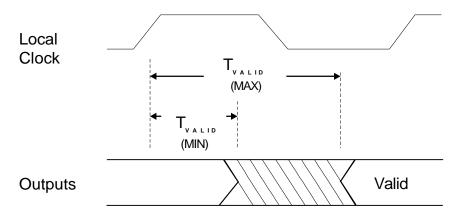
Figure 6-1. PCI 9050 Local Output Delay
