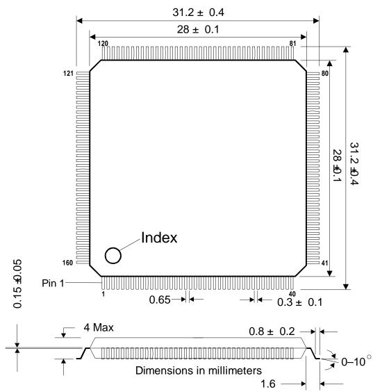
Figure 7-1. Package Mechanical Dimensions
