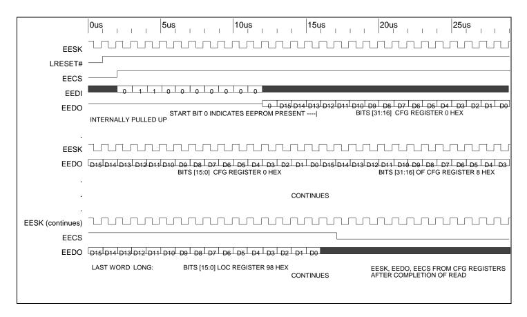
Timing Diagram 8-1. Initialization from Serial EEPROM
