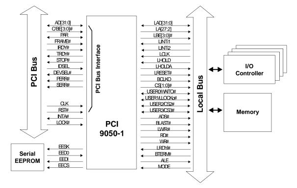
Figure 7-2. PCI 9050-1 Block Diagram
